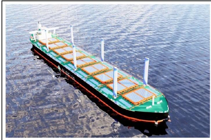
Figure 30: Rendering of the retrofitted bulk carrier with PV system installed [31]
