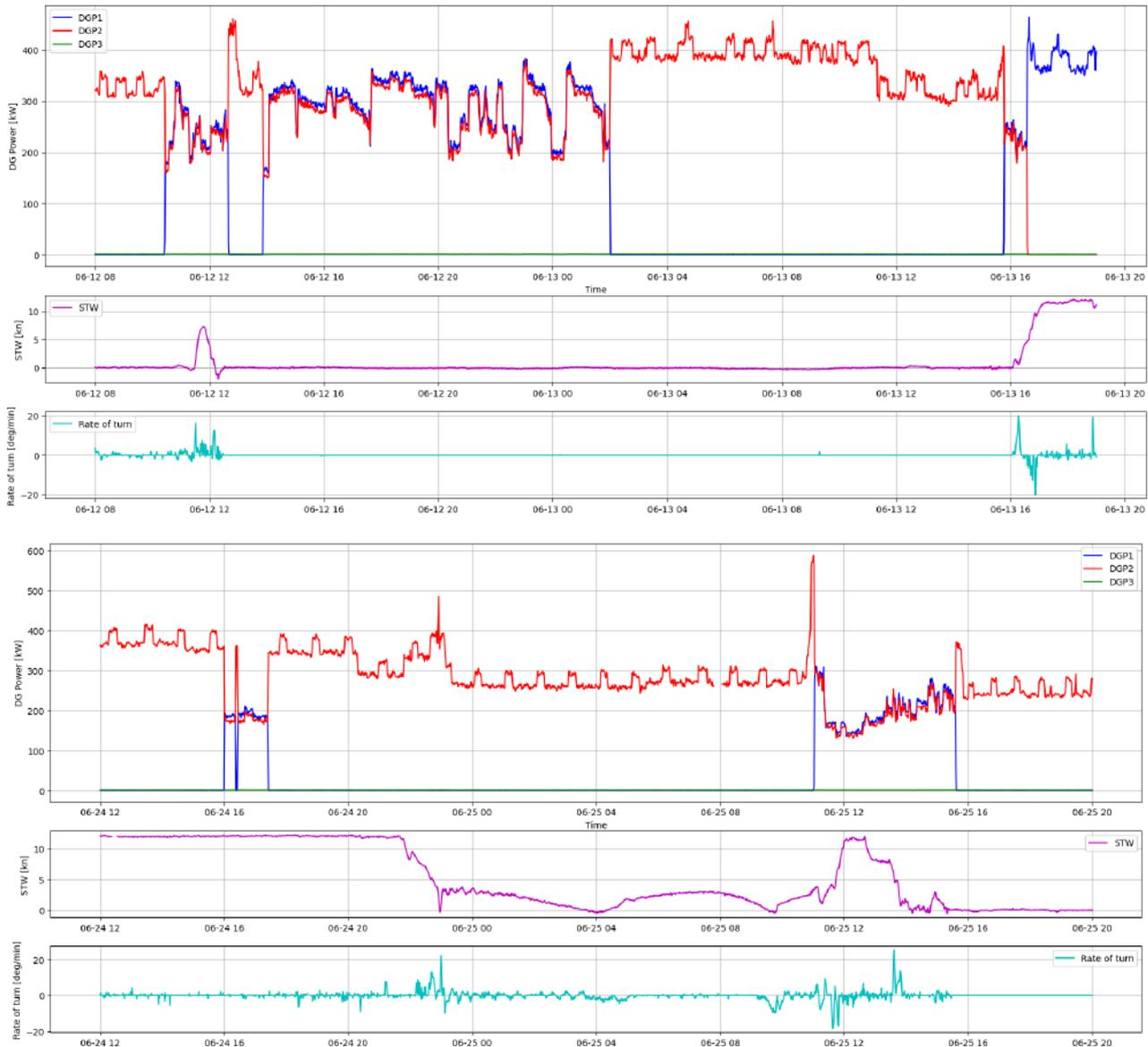
Figure 9: Time histories of DG Power, STW, and Rate of Turn during Parallel Operation Intervals with shared time axis.
